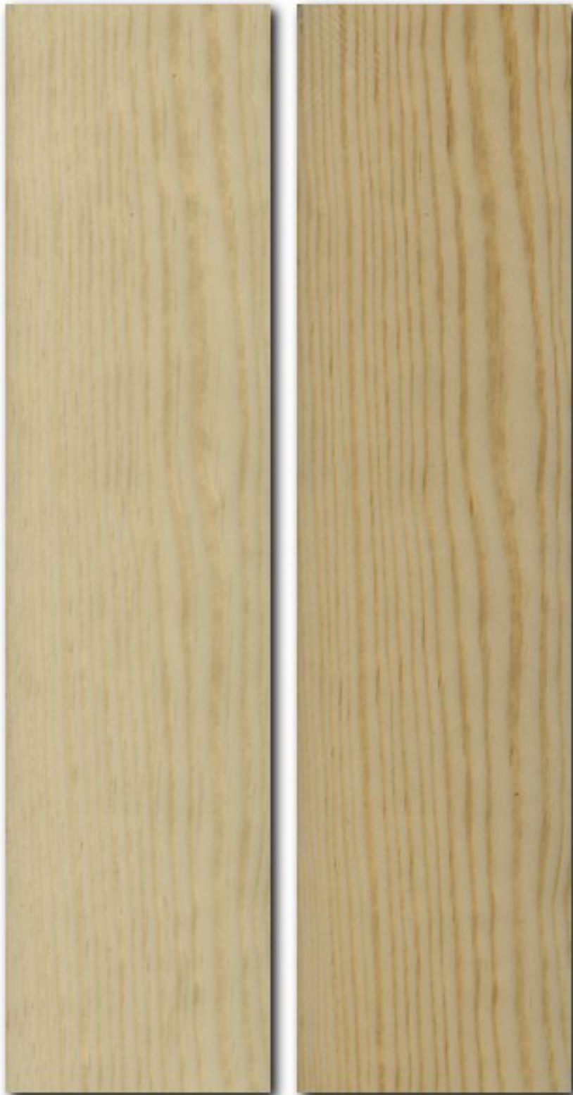
Figure 2: Sample 2 – Pine wood coated with KaWaTech HMS9 - unweathered (left), after 1 year natural weathering (right)
