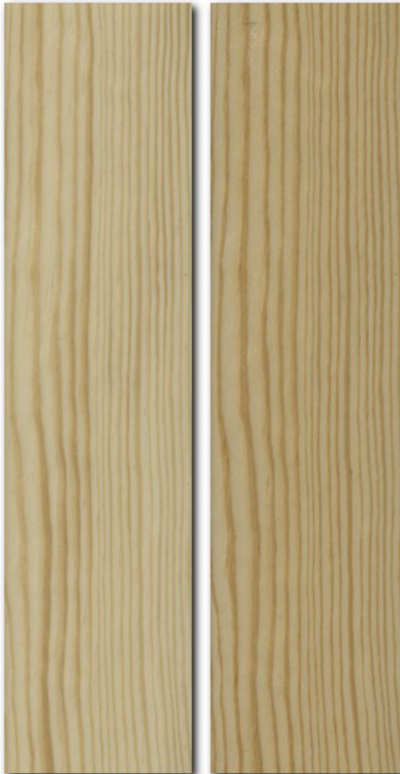
Figure 1: Sample 1 – Pine wood coated with KaWaTech HMS9 - unweathered (left), after 1 year natural weathering (right)
